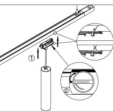
Switch to "OFF" aligned with the "►" at first, put the adaptor into the track.
